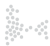
Beeswarm It emphasizes individual points in a distribution instead of binning them like a histogram.
