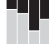
Mosaic Plot Also known as a Marimekko diagram, this chart uses the width and height of rectangles to represent separate variables. It can be useful to represent multidimensional data.
