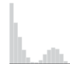
Histogram It looks like a bar chart, but it reads differently. The baseline is continuous instead of discrete categories, which allows one to see distributions.
